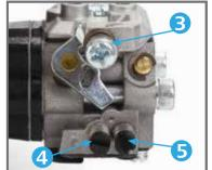
**Adjustment:** A general starting point is 1.1 turns out for the low speed needle (See No.4), and 1.5 turns out for the high speed needle (See No.5).
